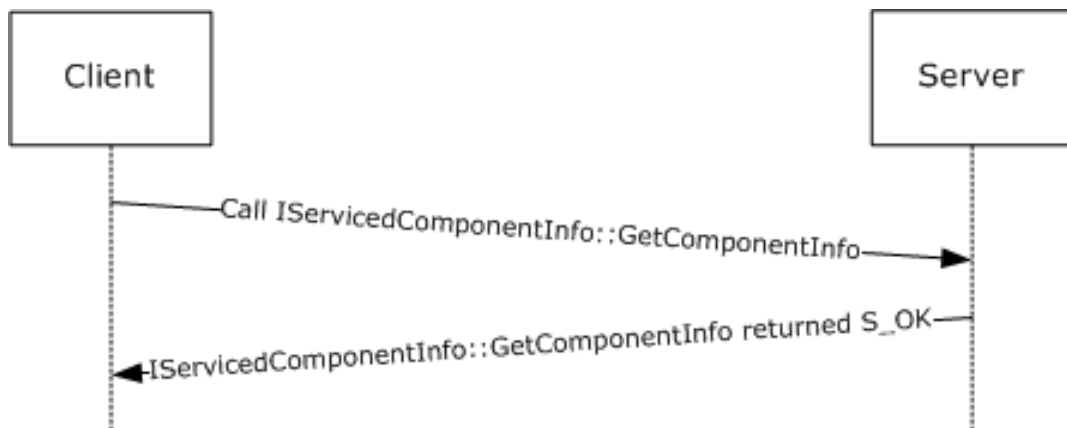
Figure 4: Call sequence for determining server object identity
