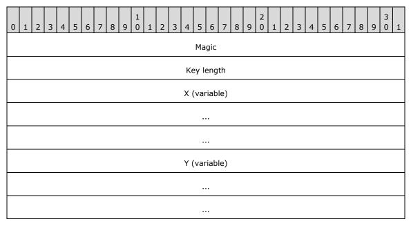
**Magic (4 bytes)**: A 32-bit unsigned integer encoded in **little-endian** format, representing the **ECDH** field parameters. The following values are valid.
