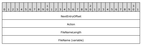
NextEntryOffset (4 bytes): The offset, in bytes, from the beginning of this structure to the subsequent FILE\_NOTIFY\_INFORMATION structure. If there are no subsequent structures, the NextEntryOffset field MUST be 0. NextEntryOffset MUST always be an integral multiple of 4.
