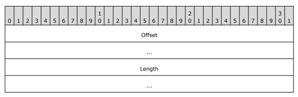
**Offset (8 bytes):** A 64-bit unsigned integer that contains a byte offset into the given file at which to start the trim request.
