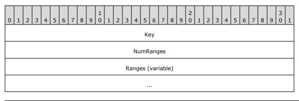
**Key (4 bytes):** This field is used for byte range locks to uniquely identify different consumers of byte range locks on the same thread. Typically, this field is used only by remote protocols such as SMB or SMB2.
