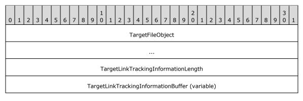
**TargetFileObject (8 bytes):** Nonzero values of **TargetFileObject** are never used in the Server Message Block (SMB) Version 2 Protocol variant of the request. This field MUST be set to zero.
