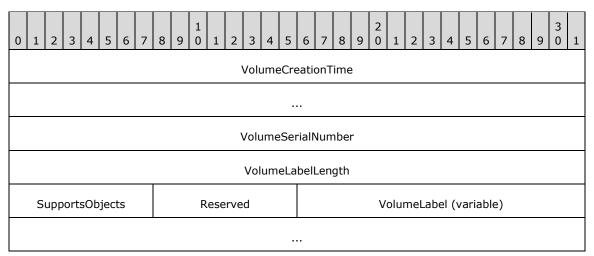
**VolumeCreationTime (8 bytes):** The time when the volume was created; see section 2.1.1. The value of this field MUST be greater than or equal to 0.
