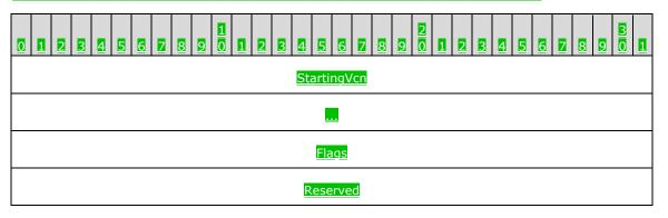
StartingVcn (8 bytes): A signed integer representing the starting VCN for which to perform the request on.
