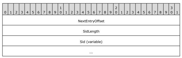
**NextEntryOffset (4 bytes):** A 32-bit unsigned integer that contains the byte offset from the beginning of this entry, at which the next FILE\_GET\_QUOTA\_INFORMATION entry is located, if multiple entries are present in a buffer. This member MUST be zero if no other entries follow this
