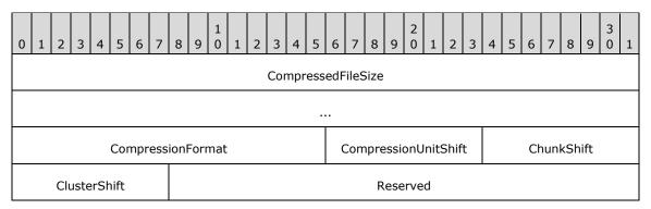
**CompressedFileSize (8 bytes):** A 64-bit signed integer that contains the size, in bytes, of the compressed file. This value MUST be greater than or equal to 0.
