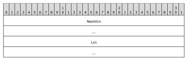
**NextVcn (8 bytes):** A 64-bit signed integer that contains the VCN at which the next extent begins. This value minus either **StartingVcn** (for the first **Extents** array element) or the **NextVcn** of the previous element of the array (for all other **Extents** array elements) is the length in clusters of the current extent.
