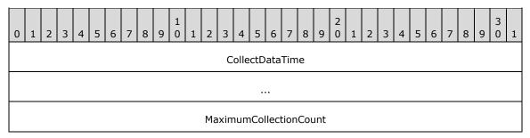
**CollectDataTime (8 bytes):** A 64-bit signed integer that MUST contain the maximum amount of time counted in 100-nanosecond intervals that will elapse before transmission of data from the client machine to the server.
