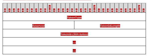
TokenType (4 bytes): A 32 bit unsigned integer that defines the type of Token that is contained within the STORAGE\_OFFLOAD\_TOKEN structure. This field MUST contain one of the following values.
