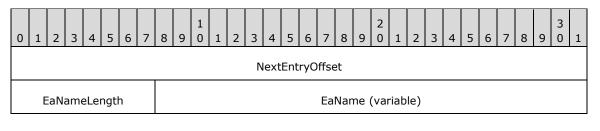
**NextEntryOffset (4 bytes):** A 32-bit unsigned integer that contains the byte offset from the beginning of this entry, at which the next **FILE\_GET\_EA\_INFORMATION** entry is located, if multiple entries are present in a buffer. This member MUST be zero if no other entries follow this one. An implementation MUST use this value to determine the location of the next entry (if multiple entries are present in a buffer).
