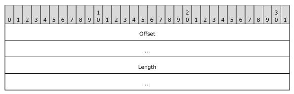
**Offset (8 bytes):** A 64-bit unsigned integer that contains a byte offset into the given file at which to start the trim request.
