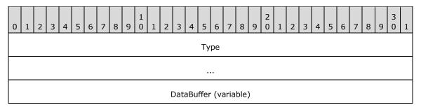
**Type (8 bytes):** A 64-bit unsigned integer value describing the type and format of the data stored in the **DataBuffer** field. The valid values for this field are:
