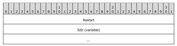
**Restart (4 bytes):** A 32-bit unsigned integer value that indicates to restart the search. This value MUST be 0x00000001 on the first call so that the search starts from the beginning of the directory on which the operation is requested. For subsequent calls, this member SHOULD be zero so that the search resumes at the point where it stopped.
