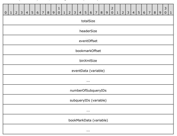
**totalSize (4 bytes):** A 32-bit unsigned integer that contains the total size in bytes of this structure, including the header.
