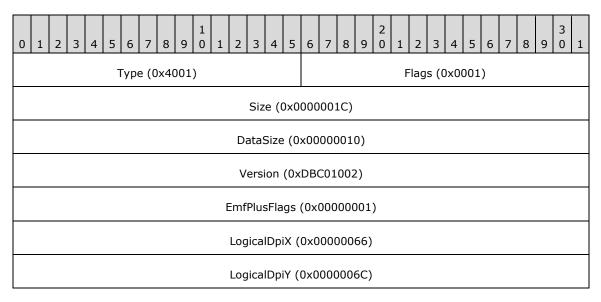
**Type (2 bytes):** 0x4001 identifies this record type as an EmfPlusHeader.
