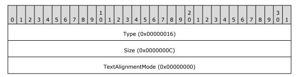
**Type (4 bytes):** 0x00000016 identifies this EMF record type as EMR\_SETTEXTALIGN.
