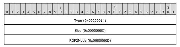
**Type (4 bytes):** 0x00000014 identifies the record type as EMR\_SETROP2.
