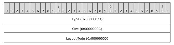
Type: 0x00000073 identifies this record type as EMR\_SETLAYOUT.
