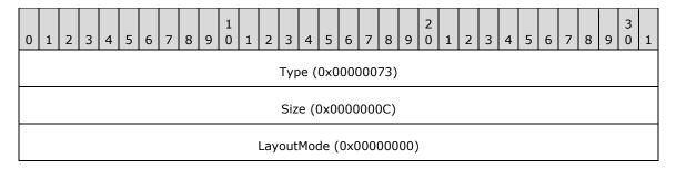
**Type (4 bytes):** 0x00000073 identifies this record type as EMR\_SETLAYOUT.
