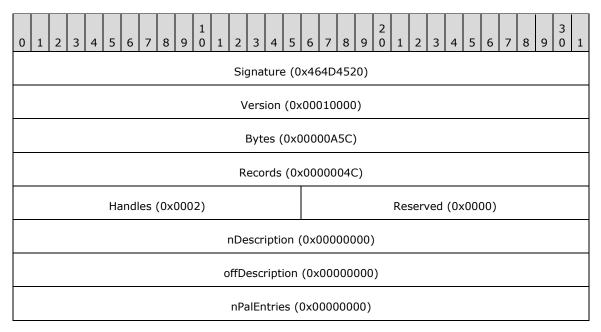
**Signature (4 bytes):** 0x464D4520 specifies the record signature, which consists of the ASCII string "EMF".
