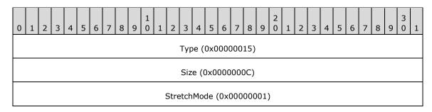
**Type (4 bytes):** 0x00000015 identifies the record type as EMR\_SETSTRETCHBLTMODE.
