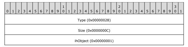
Type (4 bytes): 0x00000028 identifies this EMF record type as EMR\_DELETEOBJECT.
