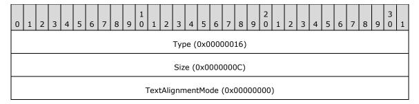
**Type (4 bytes):** 0x00000016 identifies this EMF record type as EMR\_SETTEXTALIGN.
