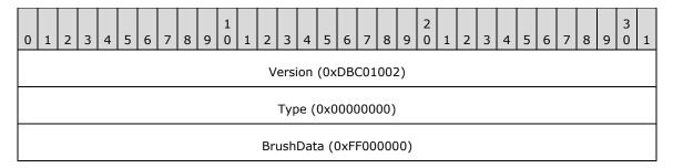
**Version (4 bytes):** 0xDBC01002 specifies the graphics version that was used to create the EmfPlusBrush object in this record.
