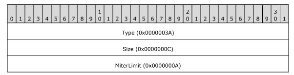
**Type (4 bytes):** 0x0000003A identifies the record type as EMR\_SETMITERLIMIT.
