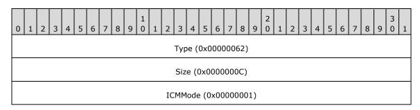
**Type (4 bytes):** 0x00000062 identifies the record type as EMR\_SETICMMODE.
