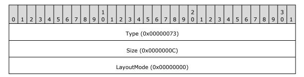
**Type (4 bytes):** 0x00000073 identifies this record type as EMR\_SETLAYOUT.
