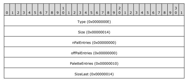
**Type (4 bytes):** 0x0000000E identifies the record type as EMR EOF.
