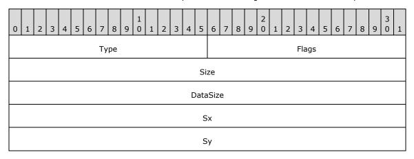
**Type (2 bytes):** A 16-bit unsigned integer that identifies this record type as EmfPlusScaleWorldTransform from the RecordType enumeration. The value MUST be 0x402E.
