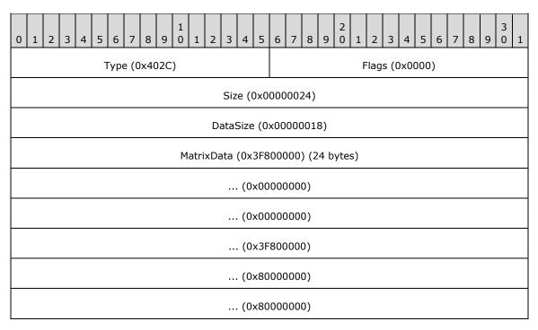
**Type (2 bytes):** 0x402C identifies the record type as EmfPlusMultiplyWorldTransform.
