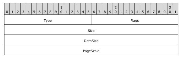
**Type (2 bytes):** A 16-bit unsigned integer that identifies this record type as EmfPlusSetPageTransform from the RecordType enumeration. The value MUST be 0x4030.
