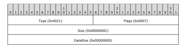
**Type (2 bytes):** 0x4021 identifies this record type as EmfPlusSetInterpolationMode.
