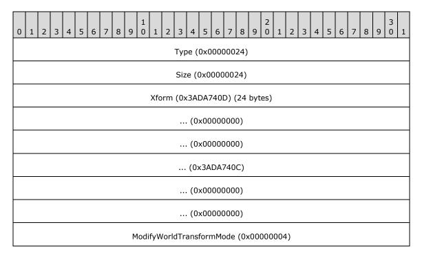
Type (4 bytes): 0x00000024 identifies the record type as EMR\_MODIFYWORLDTRANSFORM.
