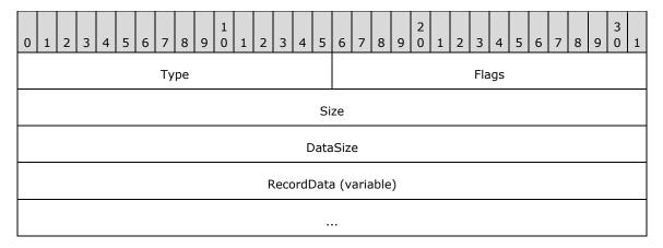
**Type (2 bytes):** A 16-bit unsigned integer that identifies the record type. The transform record types are listed below. See the table above for descriptions of these records.
