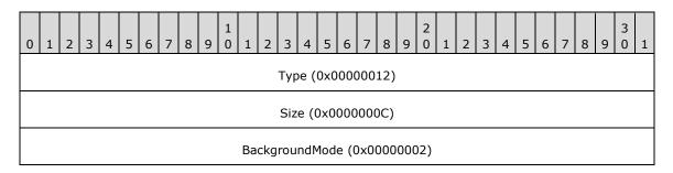
**Type (4 bytes):** 0x00000012 identifies the record type as EMR\_SETBKMODE.
