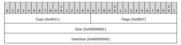
**Type (2 bytes):** 0x4021 identifies this record type as EmfPlusSetInterpolationMode.
