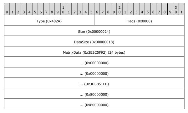
**Type (2 bytes):** 0x402A identifies the record type as EmfPlusSetWorldTransform.
