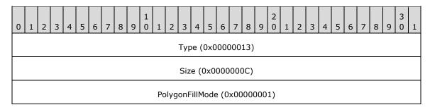
**Type (4 bytes):** 0x00000013 identifies the record type as EMR\_SETPOLYFILLMODE.
