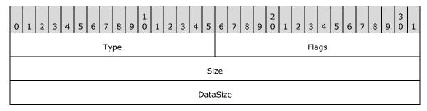
**Type (2 bytes):** A 16-bit unsigned integer that identifies this record type as EmfPlusResetWorldTransform from the RecordType enumeration. The value MUST be 0x402B.
