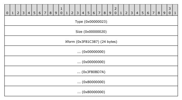
**Type (4 bytes):** 0x00000023 identifies the record type as EMR\_SETWORLDTRANSFORM.
