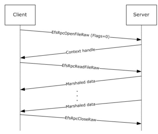
Figure 2: Message sequence for opening a file
