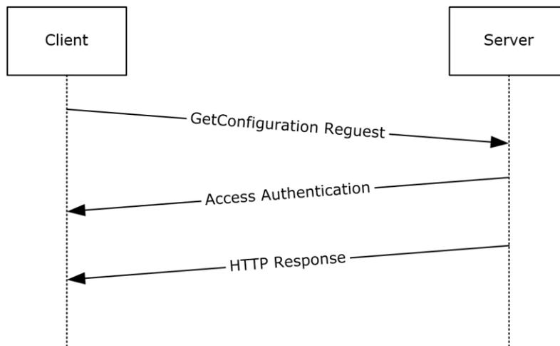
**Figure 1: Message sequence for a single GetConfiguration request**
