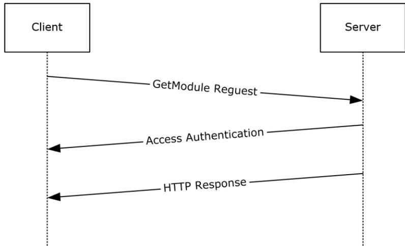
**Figure 2: Message sequence for a single GetModule request**
