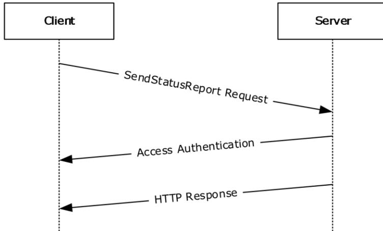
**Figure 4: Message sequence with a single SendStatusReport**
