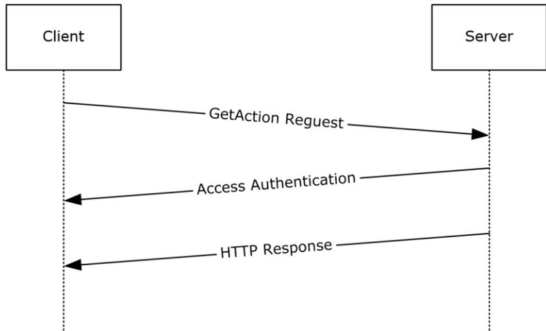
**Figure 3: Message sequence with a single GetAction request**
