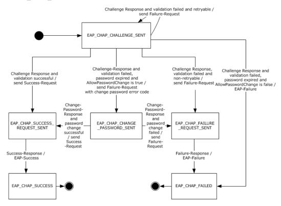
Figure 4: EAP-CHAP server state machine
