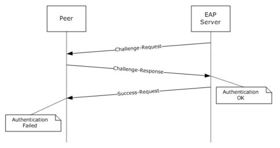
Figure 11: Authentication failure at the peer
