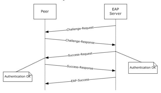
Figure 5: Peer and EAP server using successful mutual authentication
