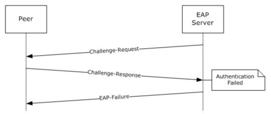
Figure 7: Authentication failure with no retry allowed
