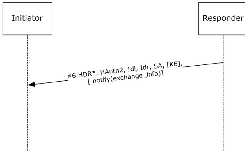
Figure 8: Quick Mode First Exchange Response packet
