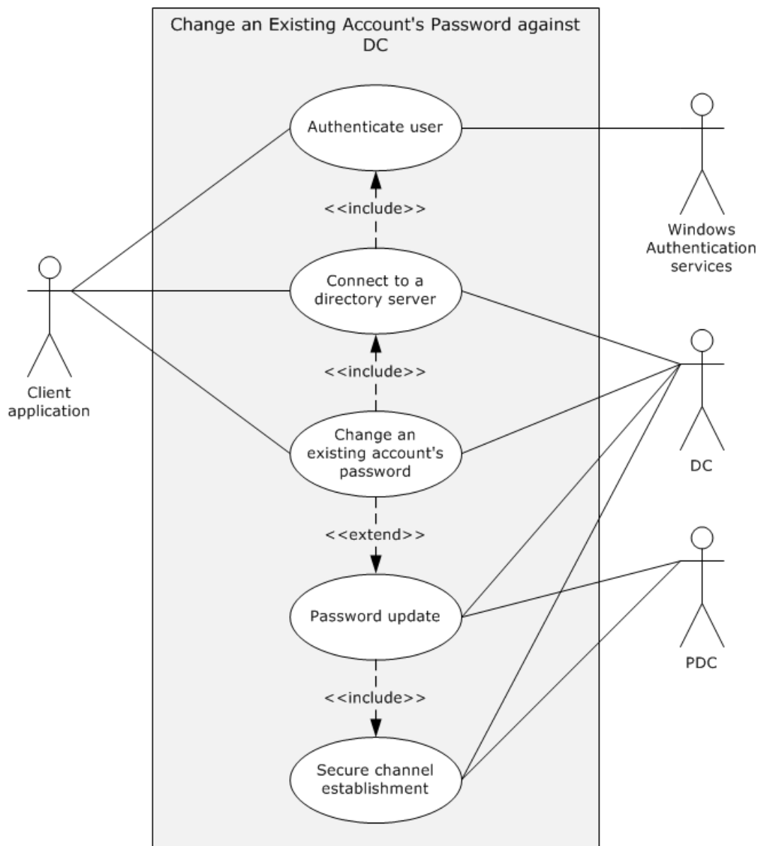
Figure 17: Use case diagram for changing the password of an existing account (DC)
