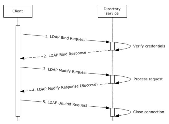
Figure 60: Message flow for extending the schema by adding an attribute to a class
