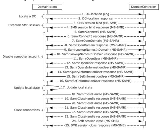
Figure 45: Message flow for unjoining from a domain
