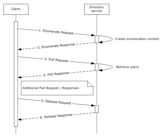
Figure 54: Communication flow for obtaining a list of user accounts by using the Web Services protocols
