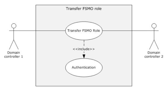
Figure 34: Use case diagram for transferring a FSMO role
