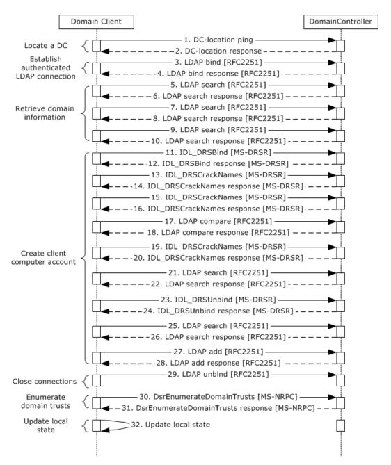
Figure 44: Message flow to join a domain by creating a new account via LDAP
