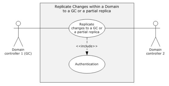
Figure 33: Use case diagram for replicating changes in a full replica to a GC or a partial replica
