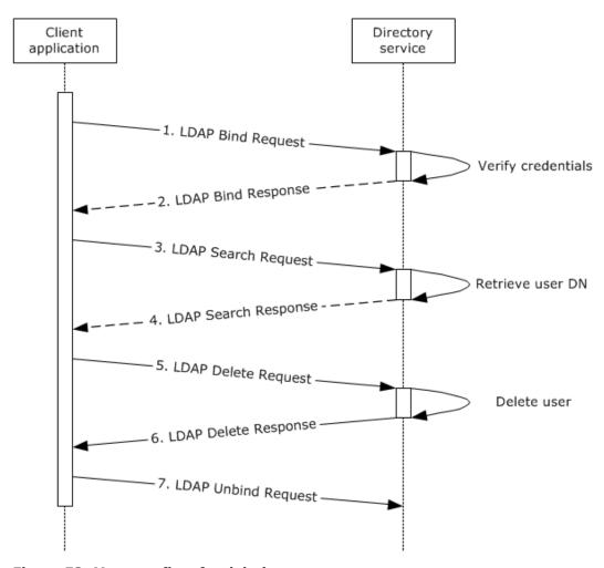
Figure 53: Message flow for deleting a user account
