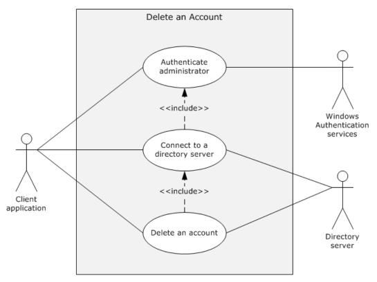
Figure 21: Use case diagram for deleting an account
