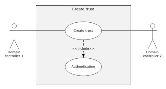
Figure 36: Use case diagram for creating a trust between domains or forests
