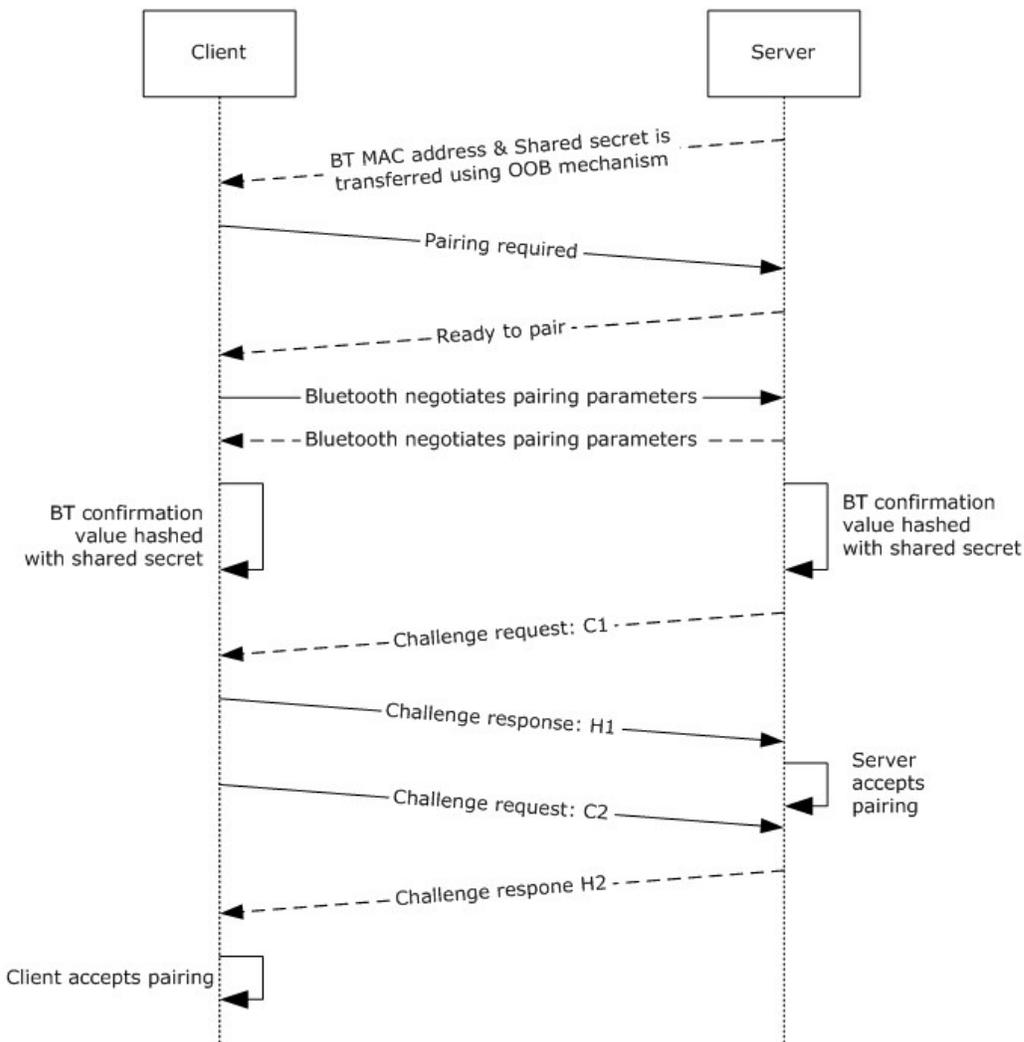
**Figure 1: Establishing a secure, authenticated Bluetooth connection**
