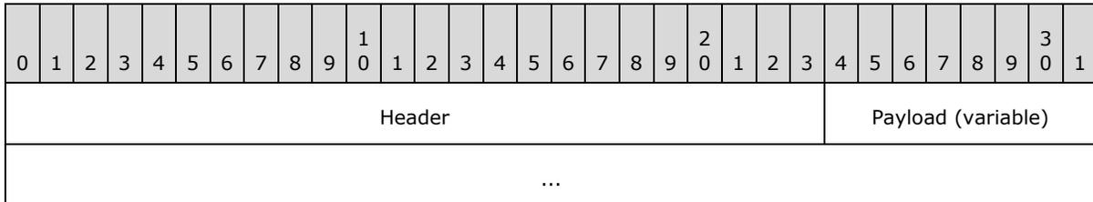
**Header (3 bytes):** This field contains the **CommonHeader** structure (section [2.2.2.1](#)). The **Id** field (**Header.Id**) of the header is set to **MessageId.Challenge** (4). The **Length** (**Header.Length**) of the header is set to the payload size of the message.
