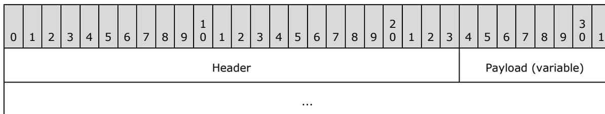
**Header (3 bytes):** This field contains the **CommonHeader** structure (section [2.2.2.1](#)). The **Id** field (**Header.Id**) is set to **MessageId.Response** (5). The **Length** field (**Header.Length**) is set to the payload size of the message.
