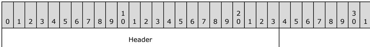
**Header (3 bytes):** This field contains the **CommonHeader** structure (section [2.2.2.1](#)). The **Id** field (**Header.Id**) is set to **MessageId.PairingRequired** (2). The **Length** field (**Header.Length**) is set to the payload size of the message. In this version of the protocol, the payload is empty (0 bytes). Future protocol versions MAY define additional message elements. This protocol version MUST ignore any payload.
