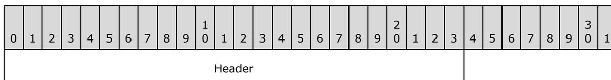
**Header (3 bytes):** This field contains the **CommonHeader** structure (section [2.2.2.1](#)). The **Id** field (**Header.Id**) is set to **MessageId.ReadyToPair** (3). The **Length** field (**Header.Length**) is set to the payload size of the message. In this version of the protocol, the payload is empty (0 bytes). Future protocol versions MAY define additional message elements. This protocol version MUST ignore any payload.
