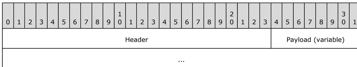
**Header (3 bytes):** This field contains the **CommonHeader** structure (section [2.2.2.1](#)). The **Id** field (**Header.Id**) is set to **MessageId.ProtocolError** (1). The **Length** field (**Header.Length**) is set to the payload size of the message. The payload consists of the **MessageId** (section [2.2.1.1](#)) of the message that was not recognized by the receiver.
