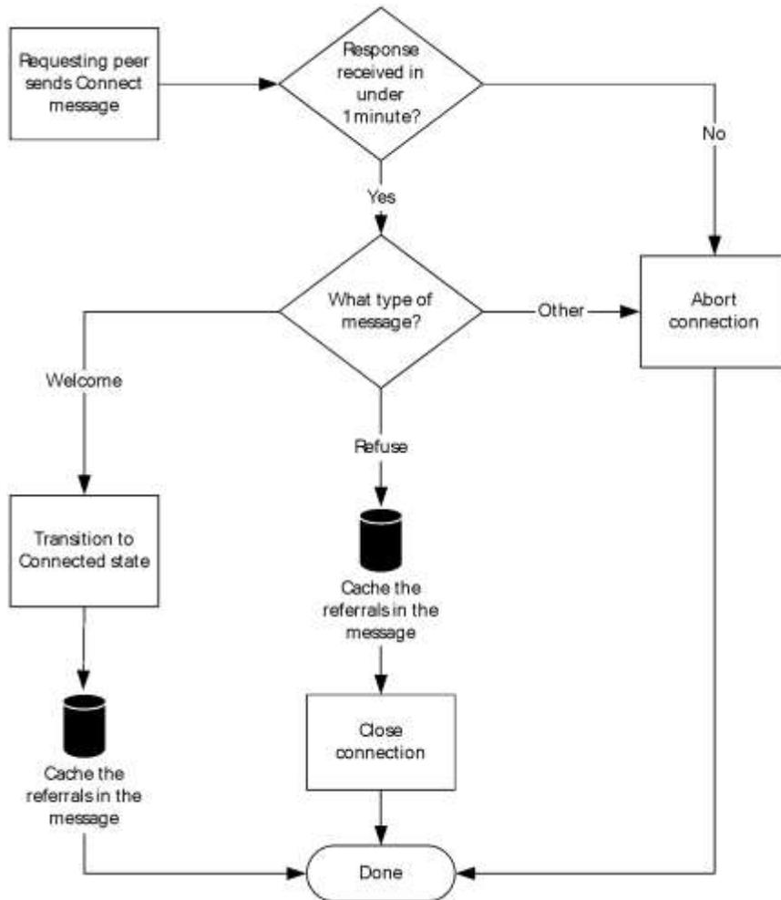
**Figure 7: Flow chart of requesting node's connection process**
