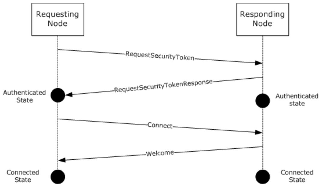
**Figure 6: Neighbor connection handshake using password-based security**
