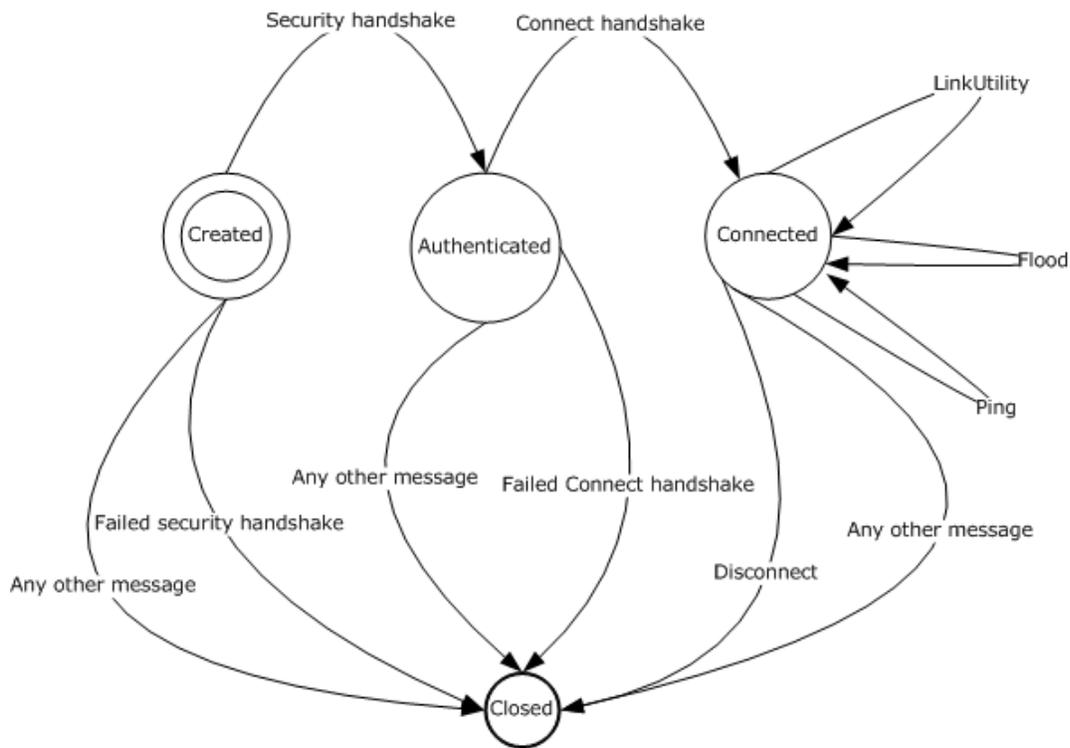
**Figure 8: State transitions of node during connection process**
