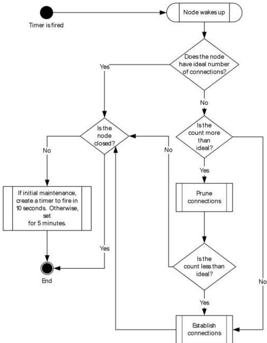
**Figure 4: Flow chart of the maintenance procedure**
