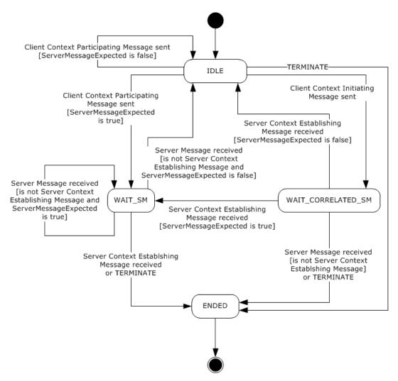
Figure 7: State diagram for the client role
