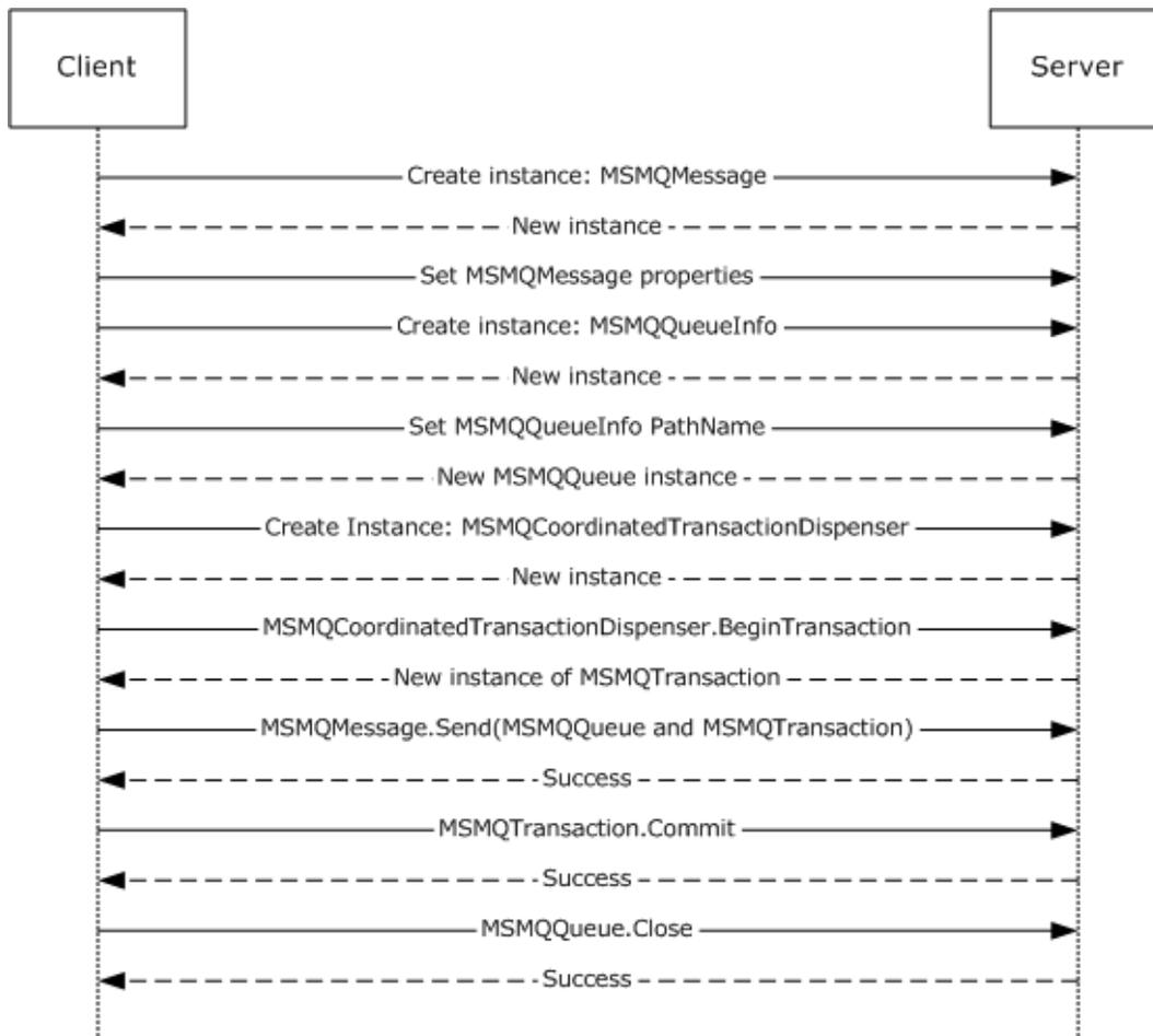
**Figure 10: Sending a message with an external transaction**
