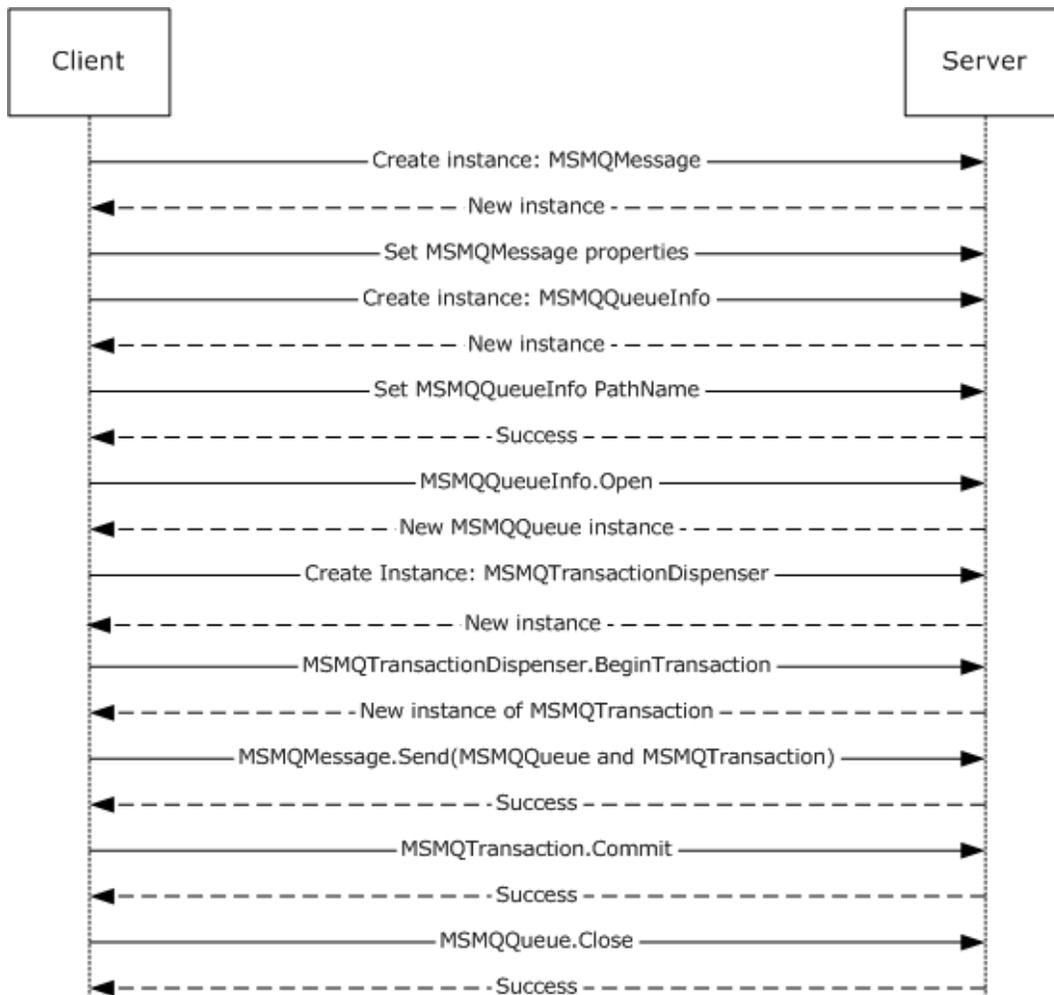
**Figure 9: Sending a message with an internal transaction**
