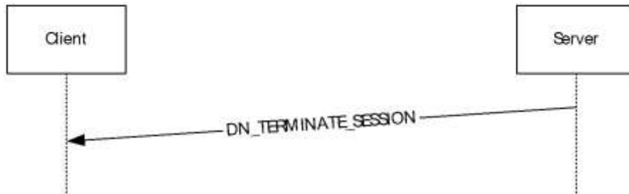
Figure 12: Client/server disconnect sequence
