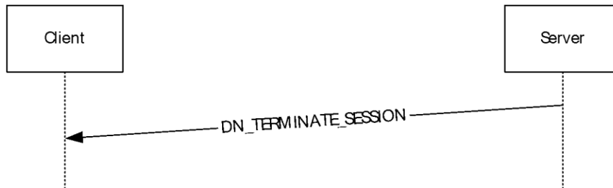
Figure 12: Client/server disconnect sequence
