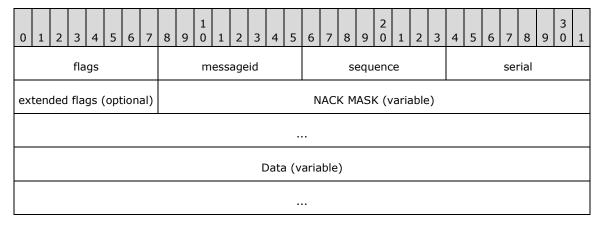
**flags (1 byte):** A bitmask that contains values from the following table that are combined using the bitwise OR operation.
