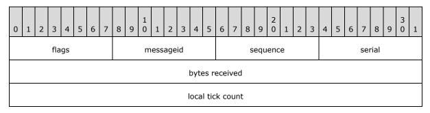
**flags (1 byte):** A bitmask that contains values from the following table that are combined using the bitwise OR operation.
