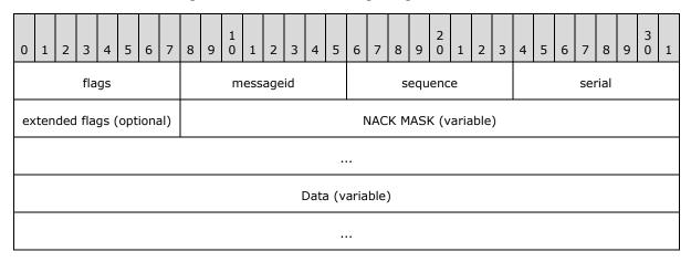
**flags (1 byte):** A bitmask that contains values from the following table that are combined using the bitwise OR operation.
